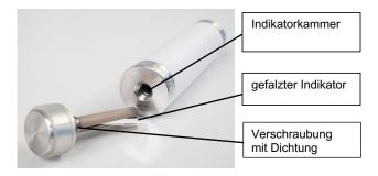
At the end of the program, the indicator is removed from the test specimen and the color change is assessed. The indicator is self-adhesive. To do this, the carrier layer is peeled off at the punching and the indicator is glued in for documentation.
